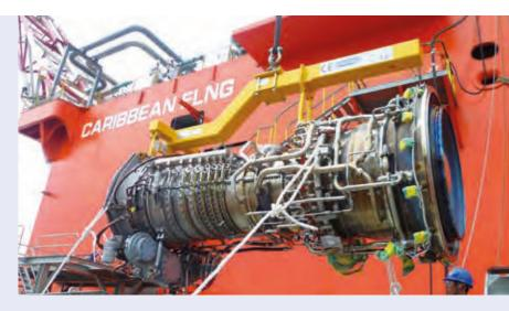
LNG. Remarkable detail: this lightweight, high-performance unit is fixed with only 2 bolts.
