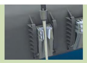
As a simpler and safer method meaning less intervention (no divers are needed), FAST™ can be applied in heavier wave and windier weather conditions than ever previously thought possible. Its design is uniform for each riser and easy to modify, making each pull-in quicker, requiring less equipment and manpower onboard, reducing overall installation costs.
